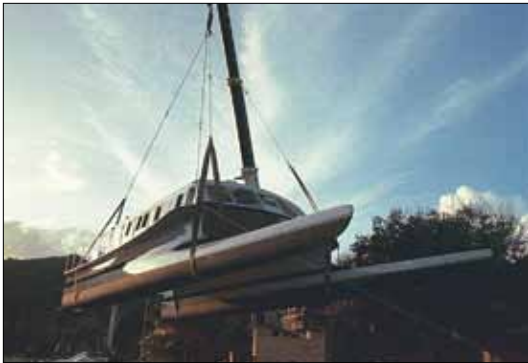
Still another market successfully exploited by Gold Coast is the passenger-carrying powercat, which—thanks to GC’s patented wave-piercing hull designed by Hatfield ( above left and left )—has proved to be a near-perfect vehicle for fast, fuel-efficient, inter-island travel. The ride quality is highly regarded, with written testimonials from experts to prove it. Above right —Spirit of Kauai, a custom GC sailing cat, scoots along under power alone.
