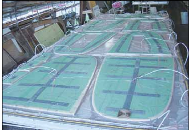
Wood-epoxy construction was the order of the day, for years, at Gold Coast. But the company made a concerted effort to gain expertise in closed molding composites, which is how GC now builds all its boats. Here we see a 50'/15.2m wave-piercer hull part ( left ) and bulkheads ( right ) being resin-infused. The company's efforts to recruit, train, and retain a skilled work force have made Difede a committed activist in the still-nascent movement to improve technical marine training nationwide.
