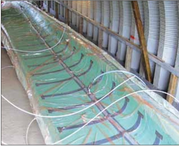
Wood-epoxy construction was the order of the day, for years, at Gold Coast. But the company made a concerted effort to gain expertise in closed molding composites, which is how GC now builds all its boats. Here we see a 50'/15.2m wave-piercer hull part ( left ) and bulkheads ( right ) being resin-infused. The company's efforts to recruit, train, and retain a skilled work force have made Difede a committed activist in the still-nascent movement to improve technical marine training nationwide.
